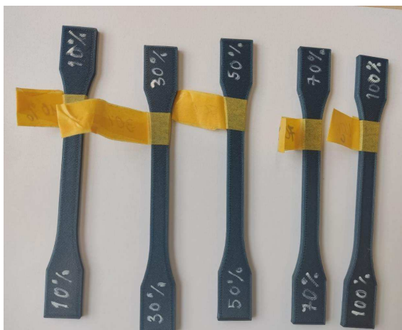
Fig. 3. PLA specimens with different infill percentages
