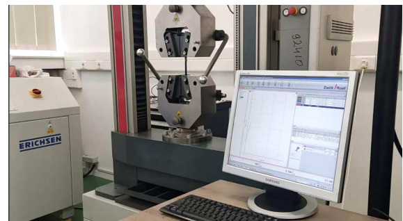
Fig. 5. Tensile test specimen
