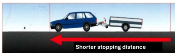
Fig. 12. Braking distance with a trailer with a braking system.
