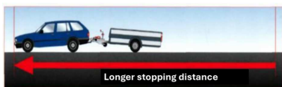
Fig. 11. Braking distance with a trailer without a braking system.
