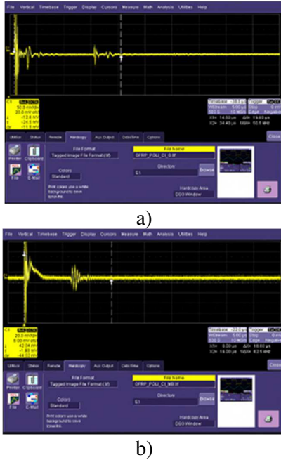
Fig. 5. Sample wave propagation for a) longitudinal waves; b) transversal waves.
