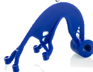
Fig 3. PLA filaments produced by UltiMaker and topology-optimized bracket fabricated.
