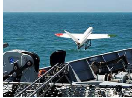
Fig. 9. World's first 3D printed aircraft automated launch from British naval ship HMS Mersey, developed by University of Southampton (UK).
