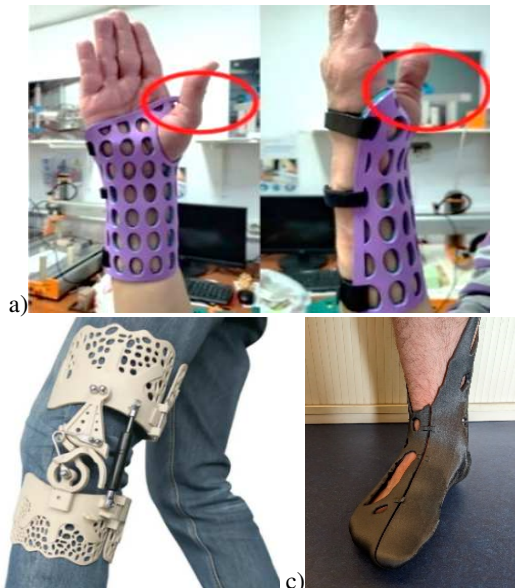
Fig. 10. Printed orthoses: a) Hand orthoses made of TPU and PLA [33], b) BioNeek system made of PEEK, c) Topology-optimized PETG-CF15 leg splint [34].
