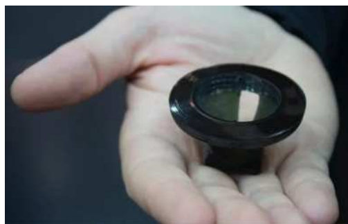
Fig. 1. World's first 3D-printed part by Chuck Hull (1983). Source: www.3dsystems.com .
