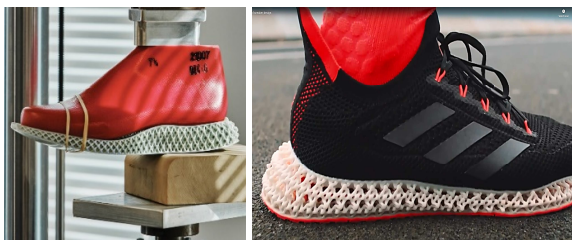
Fig. 12. MIT–Adidas collaboration on modeling running via optimal control for shoe design, integrating biomechanical modeling and additive manufacturing, enabled midsole optimization [36].
