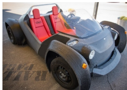
Fig. 4. Strati – the world’s first car produced using FDM technology [30].
