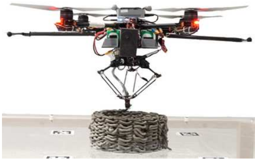
Fig. 14. Drone coordination and control used for 3D printing [38].
