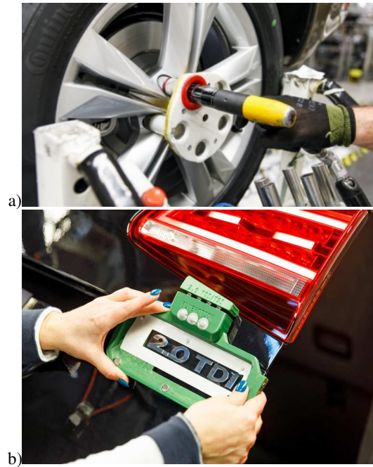
Fig. 7. Printed tools used by Volkswagen in Autoeuropa plant from Portugal: a) Wheel protection jig, b) Support used to fix the 2.0 TDI logo on liftgate.
