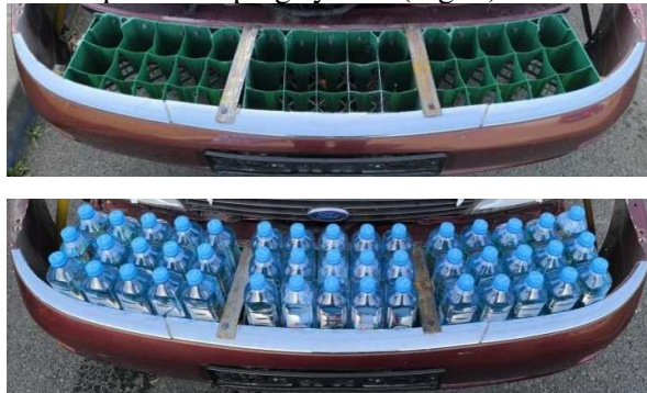
Fig. 4. Plastic frame of the damping system
