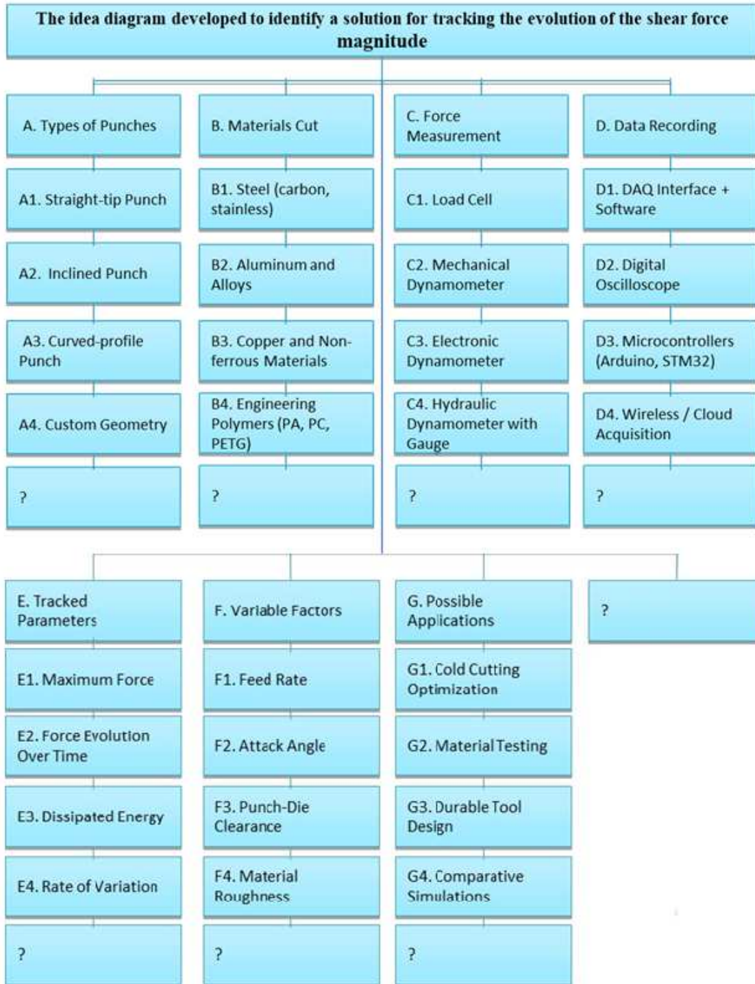
Fig. 2. The idea diagram developed to identify a solution for tracking the evolution of the shear force magnitude.
