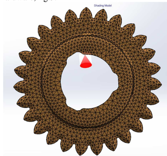
Fig.5. Finite element analysis using SolidWorks Plastics.
