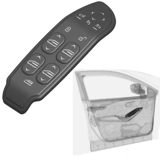
Fig. 5. 3D Part design in CATIAV5 and location of the part inside of the car
