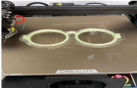
Fig. 3. Realizing personalized eyeglass frame through 3D printing
