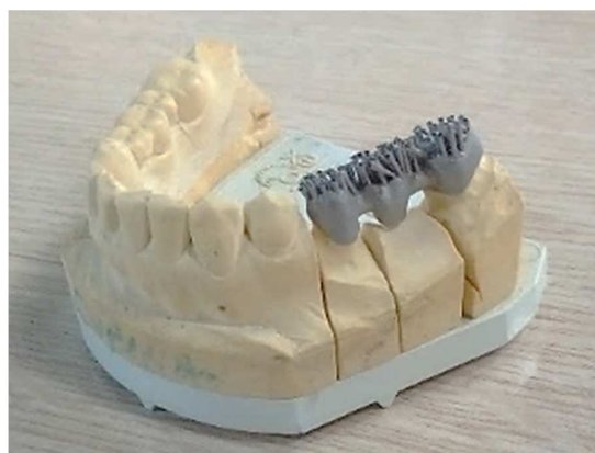
Fig. 5. Validating the results: dental bridges and test samples SLM-manufactured using the M5 set of parameters, demonstrating increased productivity (1.44 mm 3 /s).
