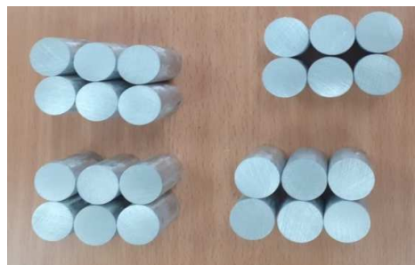
Fig. 5. The dollies used for testing
