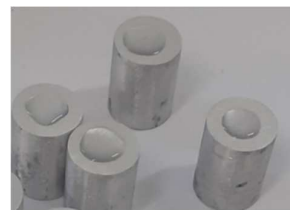
Fig. 6. The dosage of the adhesive on the surface of the dollies
