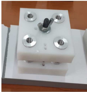
Fig. 8. The centering device with the glued dollies awaiting drying
