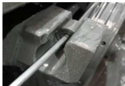
Fig. 1. Wire drawing technology; a. – wire drawing machine; b.- wire drawing die.
