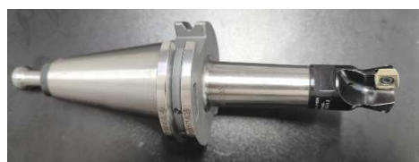
Fig. 3. The shoulder milling cutter
