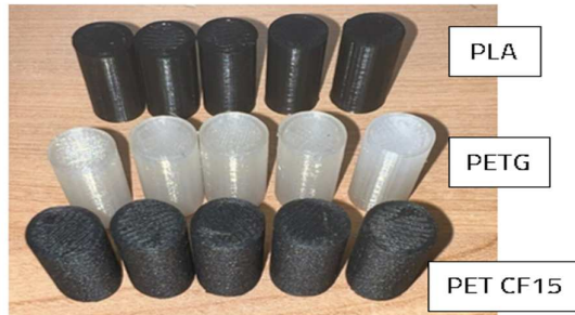
Fig. 3. Cylindrical samples according to D695 standard
