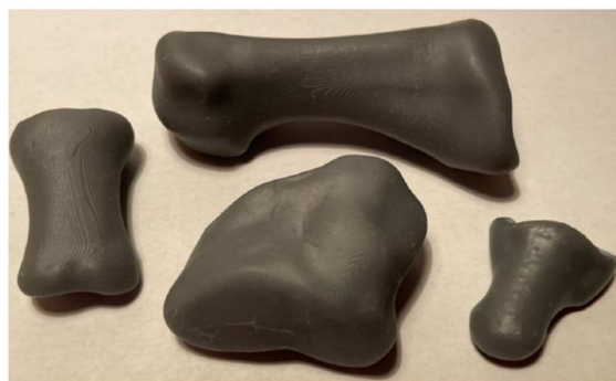
Fig. 5. Resulted bone replicas by using the SLA 3D printing method.
