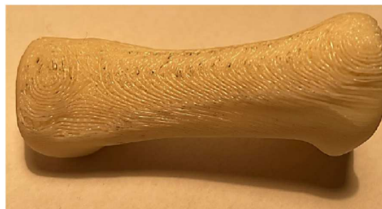
Fig. 3. Staircase effect on the 3D printed parts.
