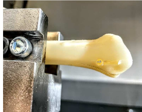
Fig. 13. Specimen after the drilling.
