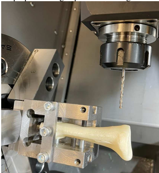
Fig. 12. Positioning of the \text{\O}3\text{mm} drill.
