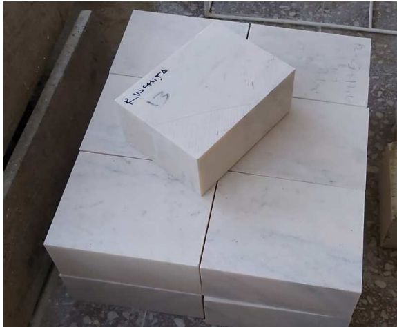
Fig. 1. Rectangular blocks of marble samples
