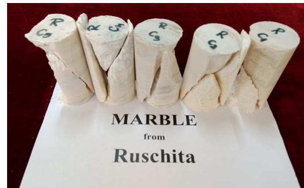
Fig.7. Failed samples in test batch 1.
