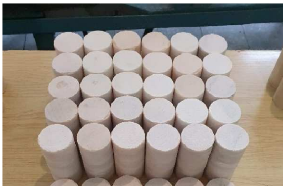
Fig. 2. Cored samples of marble
