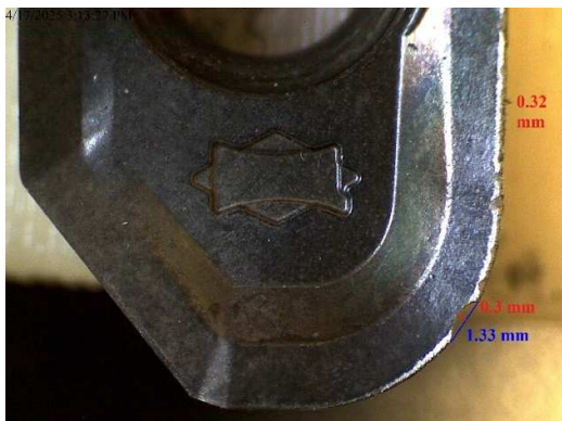
Fig. 24. Wear of DLC inserts, isometric view
