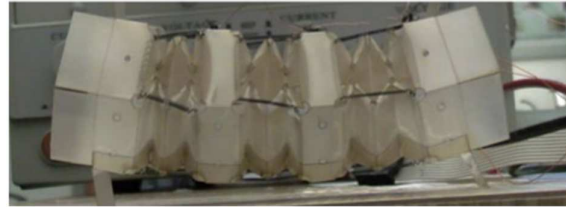
Fig. 3. Origami-inspired worm robot [7]
