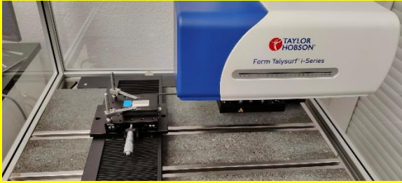
Fig. 1 Taylor Hobson Form Talysurf i-Series profilometer during measurements of Ra standard used in validation of developed simulation method of estimation of uncertainty of roughness measurements
