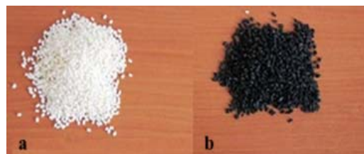
Fig. 2. a) PA6.6 pellets, b) PA6.6-30%GF.
