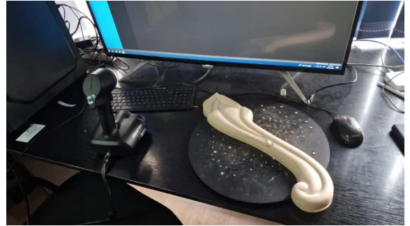
Fig. 2. 3D scanning using Go!SCAN 50 structured light scanning
