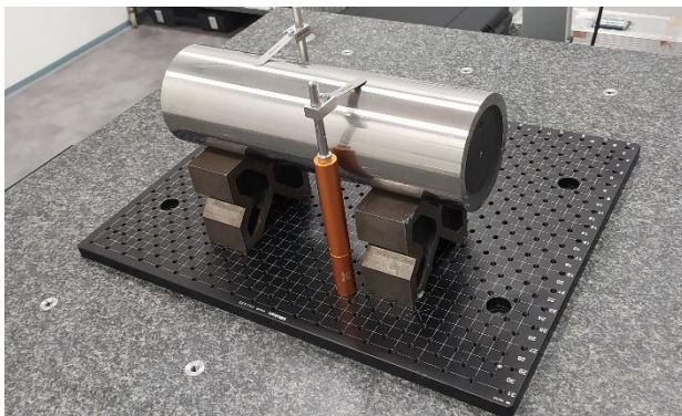
Fig. 3. Measurements of cylindrical square performed using Leitz Infinity 12.10.7 coordinate measuring machine according to guidelines of [22]
