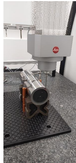
Fig. 3. Measurements of cylindrical square performed using Leitz Infinity 12.10.7 coordinate measuring machine according to guidelines of [22]
