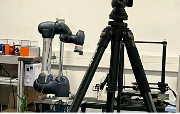
Fig. 2. Overview of the experimental setup with Doosan M1013 and C-Track 780
