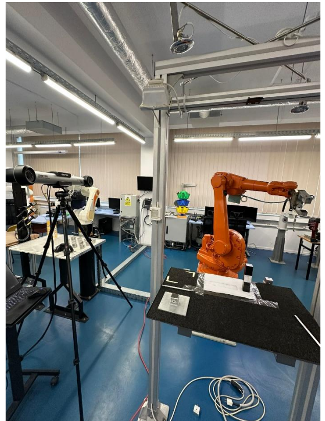
Fig. 1. Overview of the experimental setup with ABB IRB 1600 and C-Track 780
