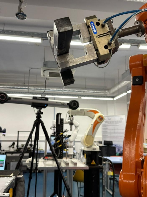
Fig. 3. Robot gripper (SCHUNK) holding test artifact
