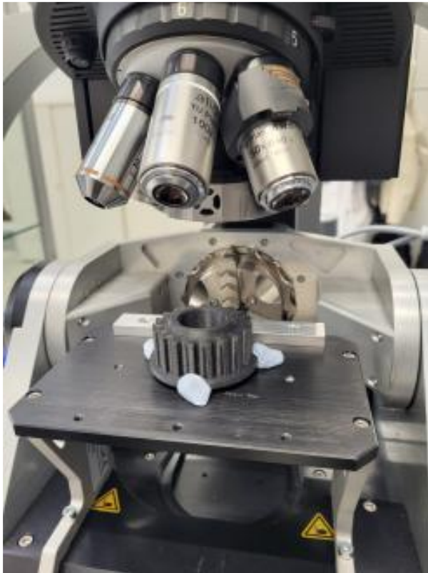
Fig. 3. Measurements of the surface fixtures with Alicona Microscope
