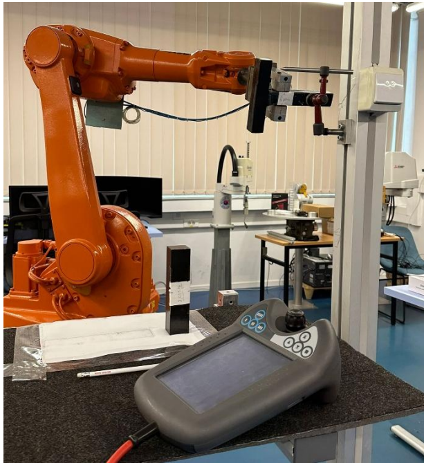
Fig. 2. Robot gripper (SCHUNK) holding test artifact Ce
