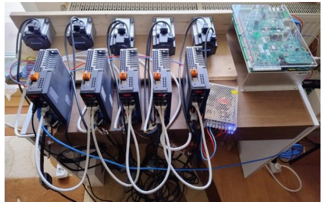
Fig. 4. Test bench for evaluating a 5 axis CNC machine
