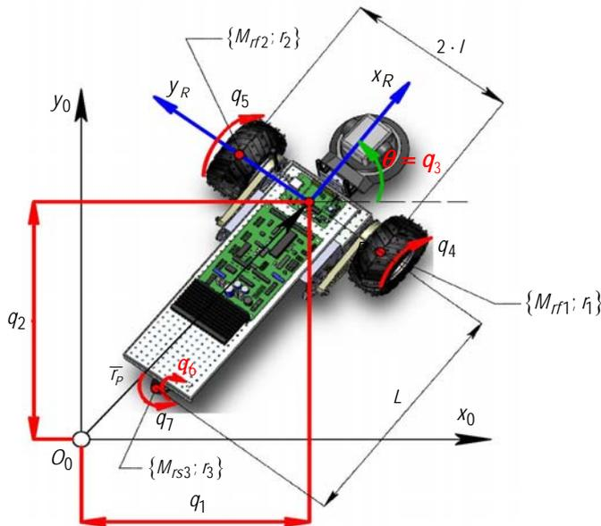
Figure 4 Independent parameters in finite displacements of RmITA mobile robot
