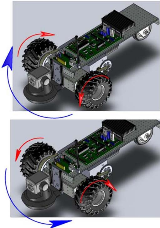
Fig.3 Orientation of the mobile structure
