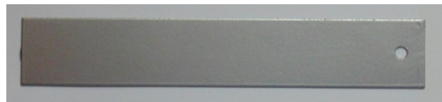
Fig. 3. Steel test tube, painted in eletrostatic field - size 150x25x1 mm.
