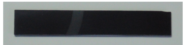
Fig. 7. Glass ceramic, EUROKERA, size 150x25x4 mm.
