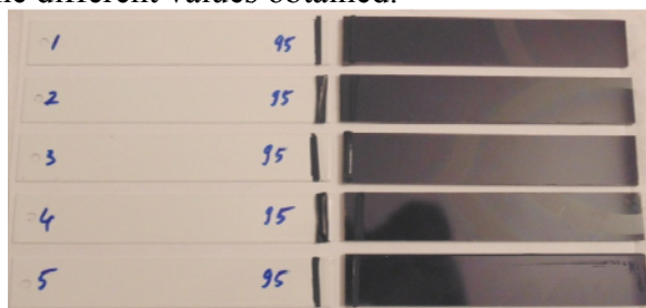
Fig. 25. Test tubes of painted material after tensile tests.
