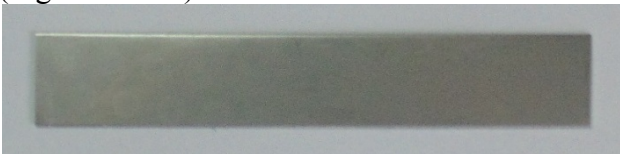
Fig. 1. Stainless steel test tube - size 150x25x1 mm.
