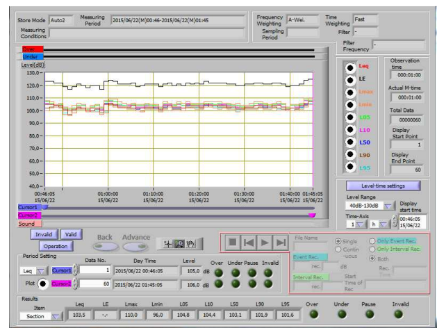
Fig. 3. The data measured at a distance of 1 m from the main source of the noise – power pump room.
