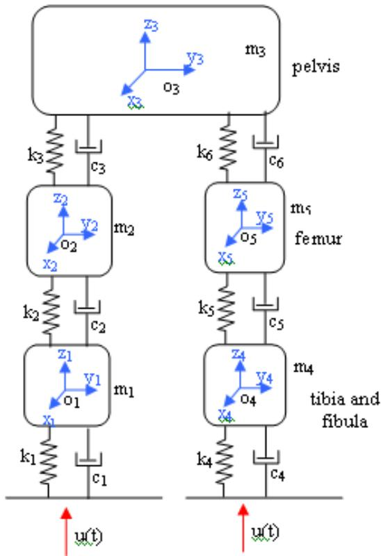
Fig. 1 Simplified mechanical models of human pelvis and legs with five degrees of mobility
