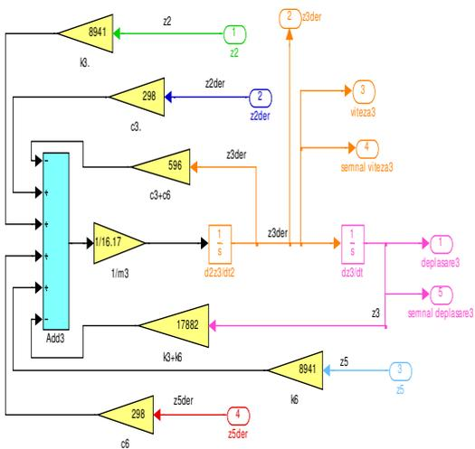
Fig. 4. Subsystem  $z_3$  5-EPP program properly
