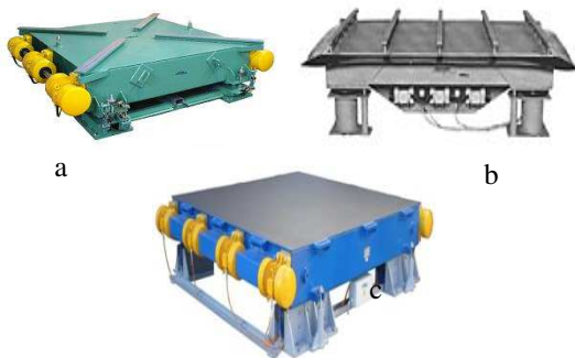
Fig. 1 a. Work table; b. Vibrating work table with vibrant guide rails; c. Vibrating work table for tamping the concrete carcasses [11].
