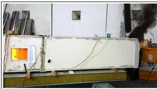
Fig. 4. Reduced scale tunnel model during experimental test (gasoline pool fire)
