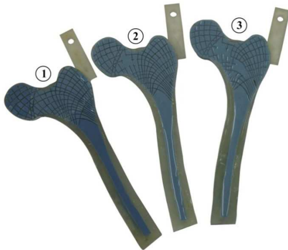
Fig.4 2D physical models: 1 – referential model; 2 – OP model with 12 trabeculae affected; 3 – OP model with 47 trabeculae affected.
