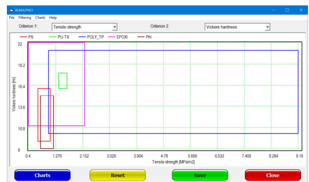
Fig. 10. Two-Dimensional map Tensile Strength vs. the Vickers hardness
