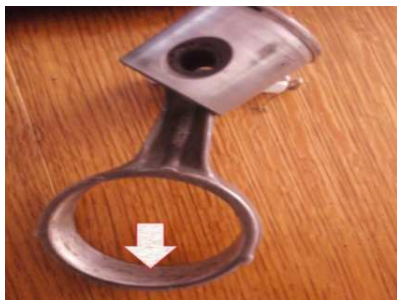
Fig. 2. Connecting rod worn due to improper lubrication
