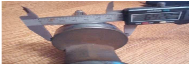
Fig. 3. Measuring the wear at the crankpin
