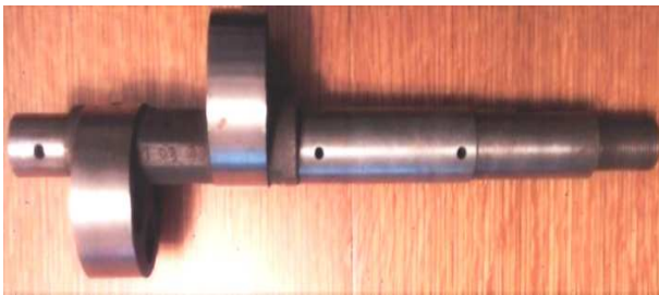
Fig.7. Eccentric shaft after metallization and finishing
