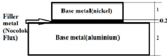
Fig. 1. The contact between base and filler metal by Nocolok Flux. Digits: 1, 0.2, and 2 are in mm.
