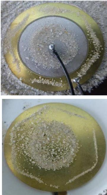
Fig. 6. Vibration mode at 8550Hz
