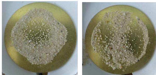
Fig. 5. 4500Hz and 5300Hz vibration modes
