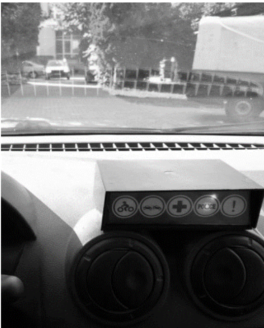
Fig.9 The display module installed in the car
