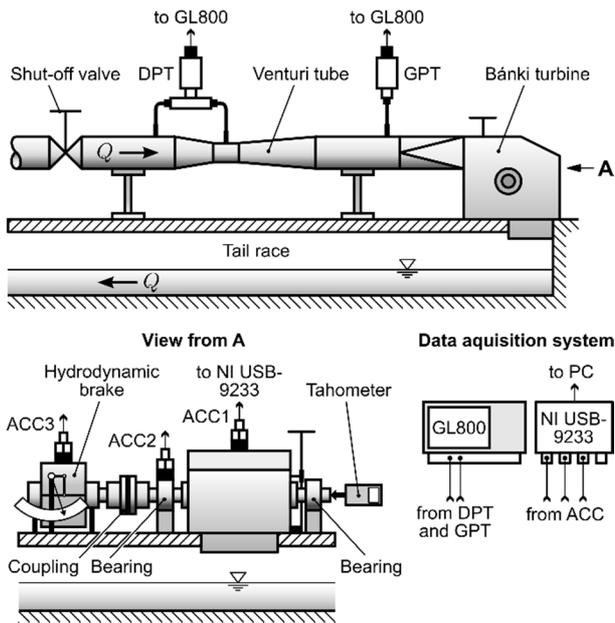
Fig. 1. Experimental installation
