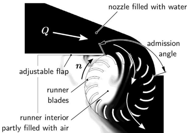
Fig. 2. Turbine cross-section and the flow inside it [8]
