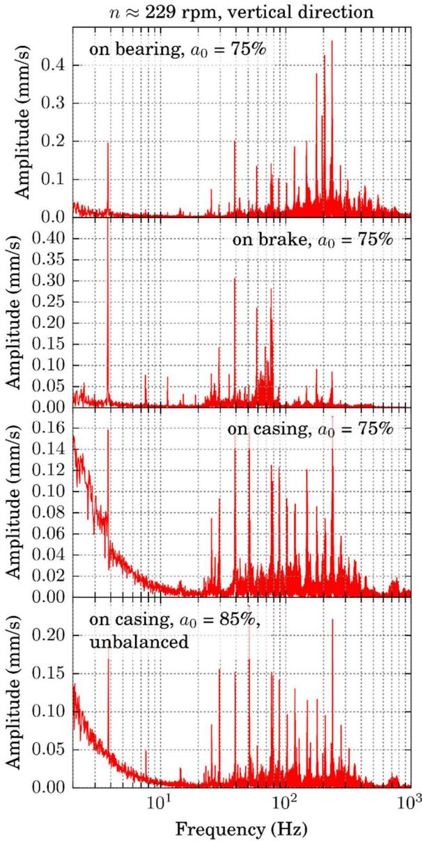
**Fig. 4.** Comparison between FFTs of vibrations measured at roughly 229 rpm in vertical direction.
