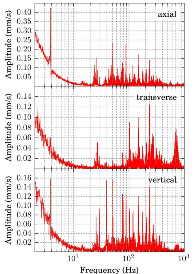
**Fig. 3.** FFTs of vibrations measured at a flap opening of 75% and a runner speed of roughly 229 rpm, on top of the turbine casing.
