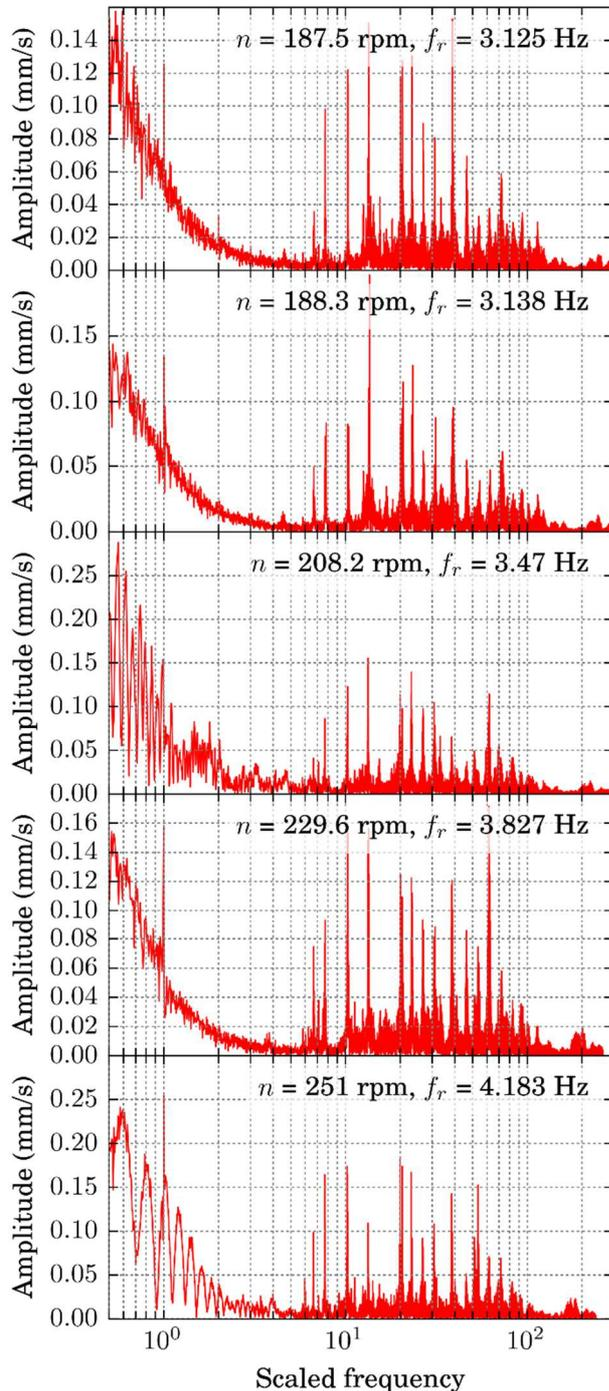
**Fig. 5.** Scaled FFTs of vibrations measured on top of the casing at different runner speeds.
