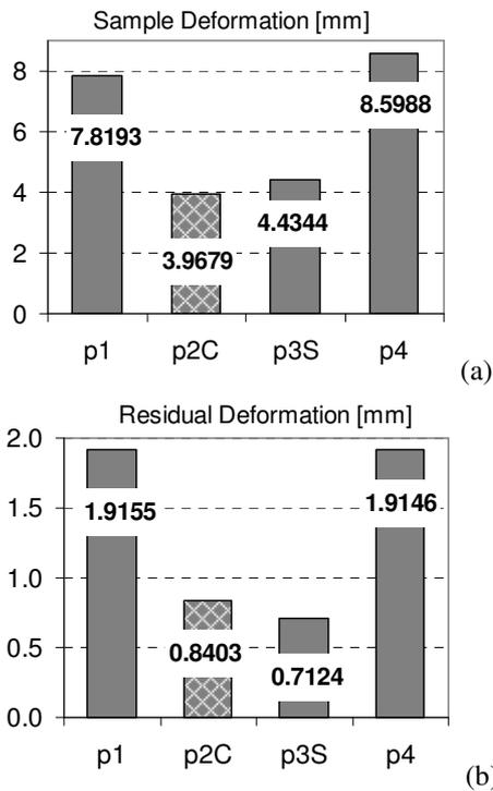
**Fig. 15.** Maximum values of the samples total deformation (a) and of the residual deformation (b) in respect with the first impact cycle - classical LDC sample was distinctively marked
