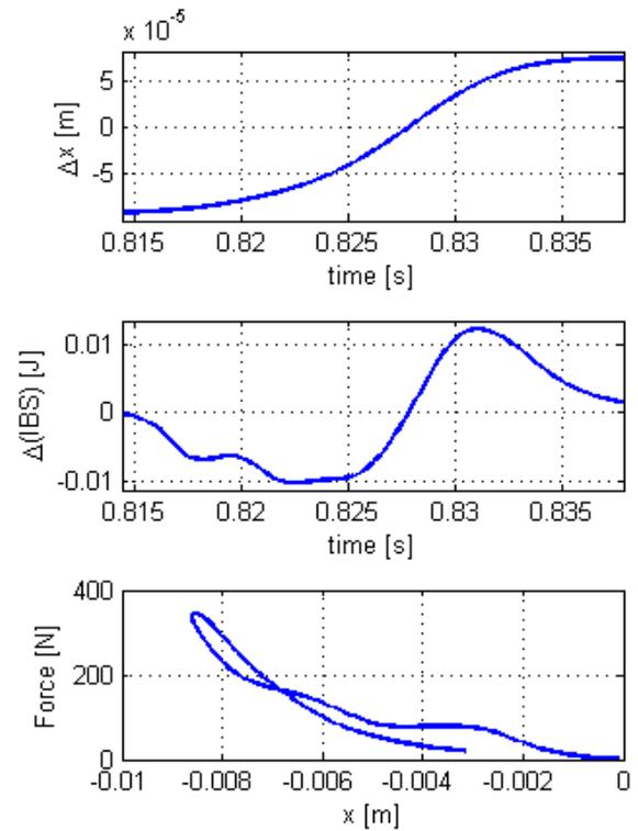
**Fig. 10.** Instantaneously evolutions of deformation and impact bending strength respectively, and the force – deformation diagram for the sample p4
