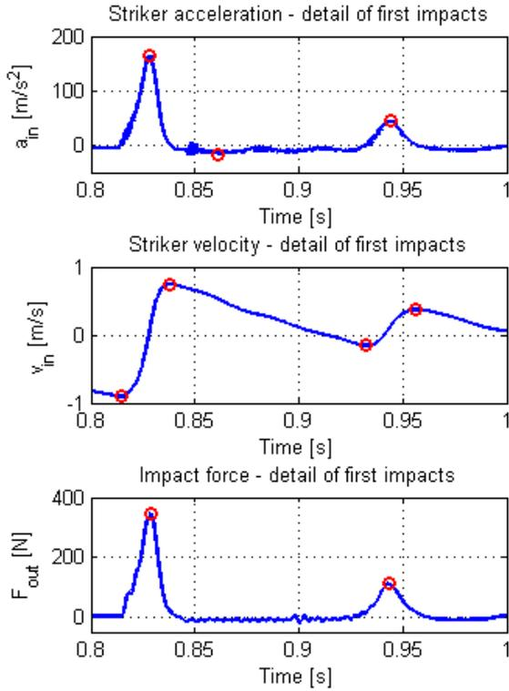
**Fig. 5.** Timed signals of acceleration, velocity and impact force acquired for the sample p4; circle symbols on graphs denote the local extremes according with first cycles
