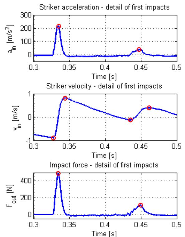
**Fig. 4.** Timed signals of acceleration, velocity and impact force acquired for the sample p3S; circle symbols on graphs denote the local extremes according with first cycles
