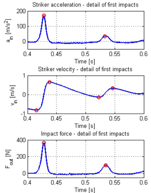
**Fig. 3.** Timed signals of acceleration, velocity and impact force acquired for the sample p1; circle symbols on graphs denote the local extremes according with first cycles
