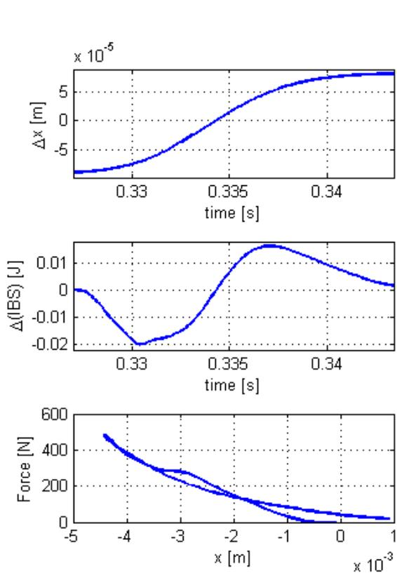
**Fig. 9.** Instantaneously evolutions of deformation and impact bending strength respectively, and the force – deformation diagram for the sample p3S
