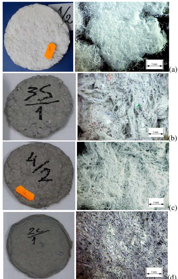
**Fig. 1.** The samples with their microphotographs of the materials used for experimental tests (reflex photo, magnification 20x): (a) sample p1, (b) sample p3S, (c) sample p4, (d) sample p2C – see text for details.
