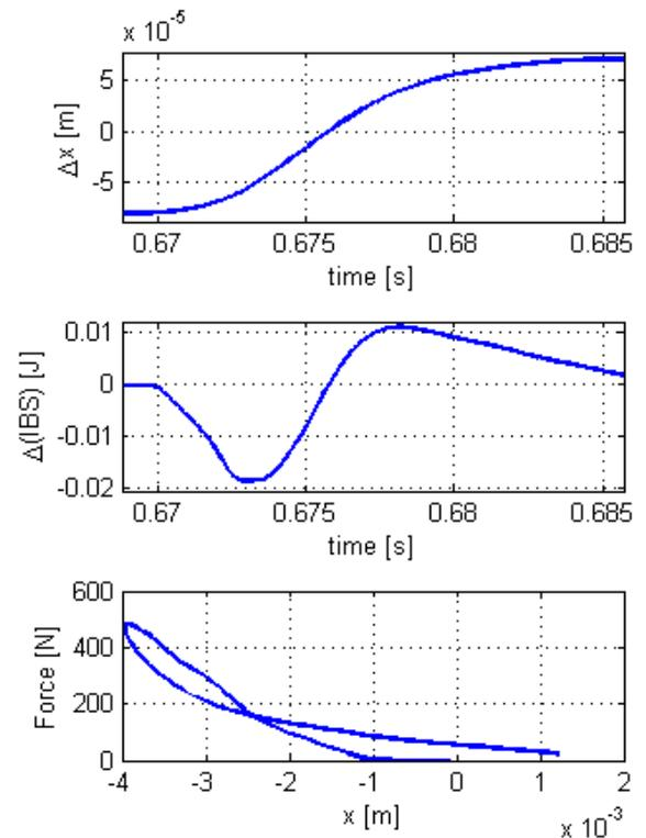
**Fig. 11.** Instantaneously evolutions of deformation and impact bending strength respectively, and the force – deformation diagram for the sample p2C
