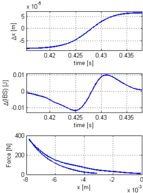
**Fig. 8.** Instantaneously evolutions of deformation and impact bending strength respectively, and the force – deformation diagram for the sample p1
