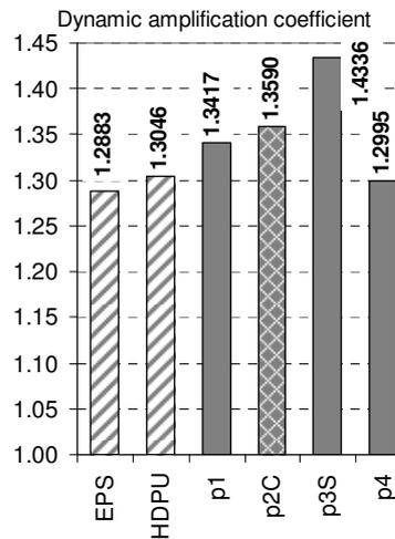
**Fig. 13.** Comparative analysis of dynamic amplification coefficient – reference samples and classical LDC samples were distinctively marked
