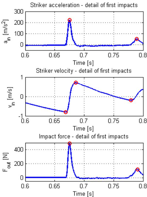
**Fig. 6.** Timed signals of acceleration, velocity and impact force acquired for the sample p2C; circle symbols on graphs denote the local extremes according with first cycles
