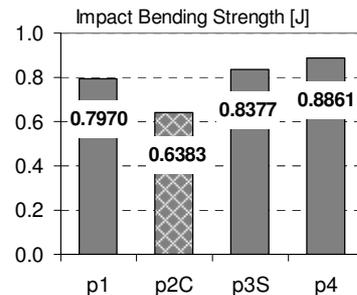
**Fig. 14.** Maximum values of the impact bending strength in respect with the first impact cycle - classical LDC sample was distinctively marked
