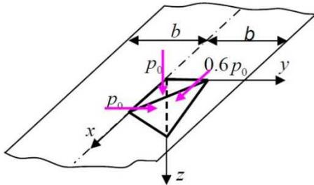
Fig. 9. The main unit efforts on the middle line of the contact strip
