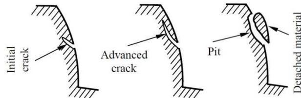
**Fig. 4.** The cracks growths on the teeth flanks
