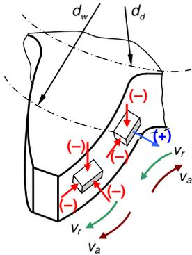
Fig. 6. The stresses distribution on the tooth flank
