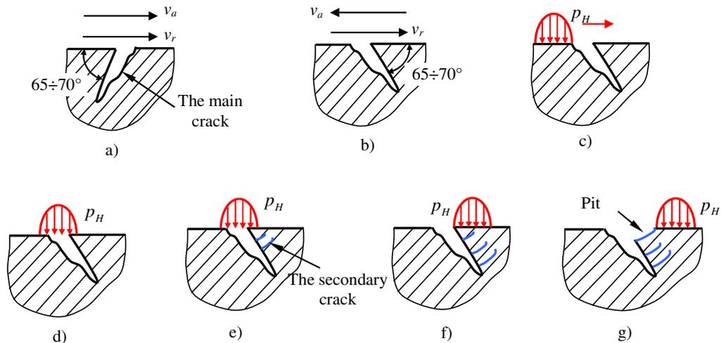
**Fig. 5.** The pitting mechanism, the main and the secondary cracks
