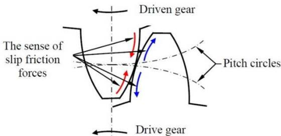
**Fig. 2.** The direction of the slip friction forces
