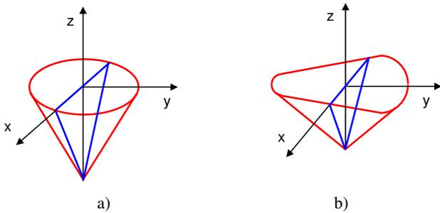
Fig. 7. The deformed stresses cone
