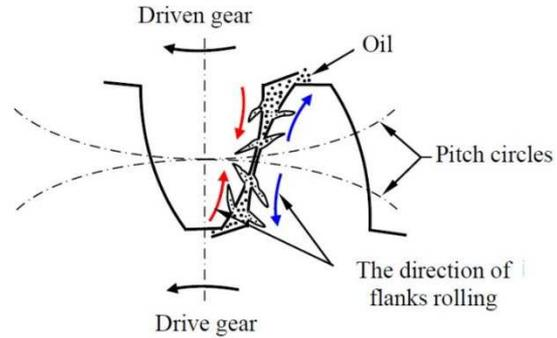
**Fig. 3.** The appearance of cracks on the surface of the teeth
