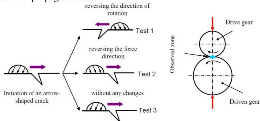
**Fig. 11.** The effect of the rotation direction and the role of the coupling elements
