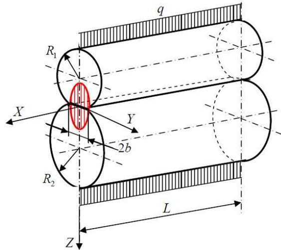
Fig. 8. Elastic contact on two-cylinder with parallel axes
