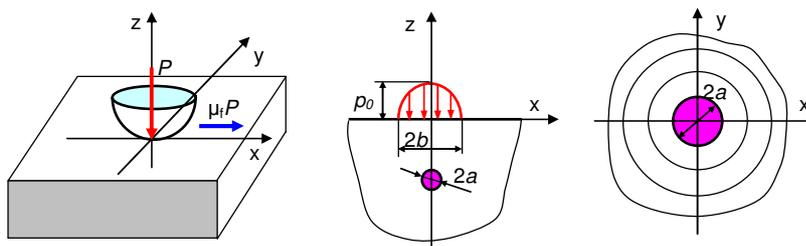
Fig. 10. The schematization of punctual hertzian contact in defective environments
