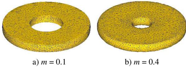
**Fig. 6.** FE simulation compressed rings at a reduction in height,  $\Delta h = 60\%$  and two values of friction factor ( $m$ )
