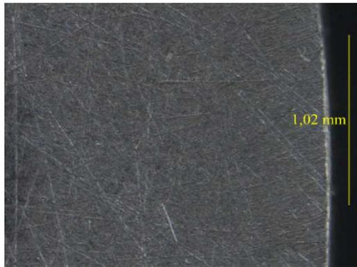
a) - Ring specimen type 1 (Ra=0.32 μm)
