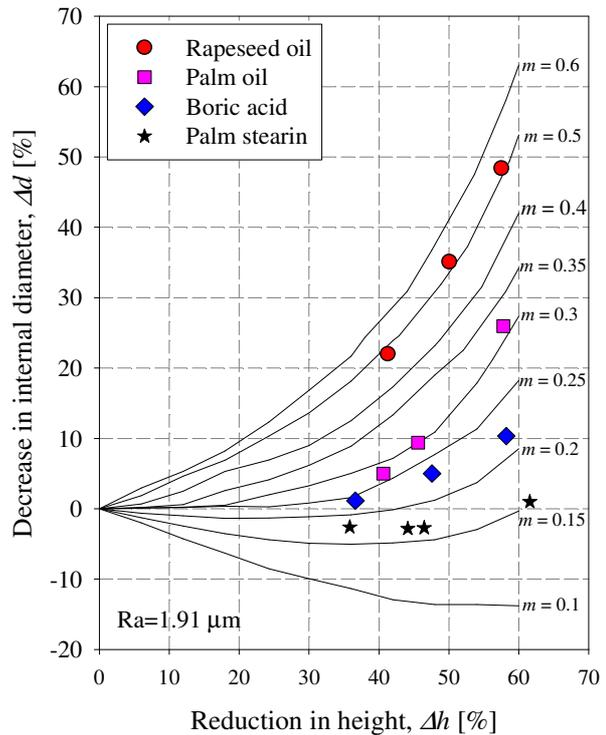
**Fig. 9.** Friction calibration curves and experimental results for the workpiece surface roughness of  $0.91 \mu\text{m}$
