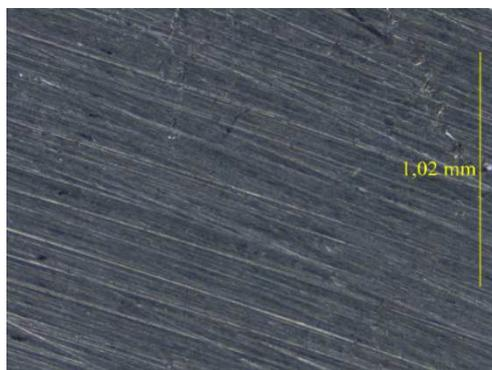
b) - Ring specimen type 2 (Ra=0.6 μm)
