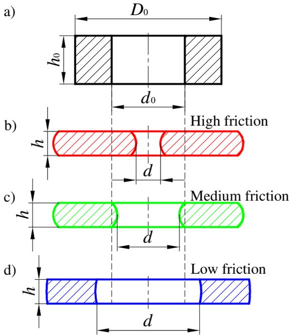
Fig. 1. Different cases of material flow during the ring compression test
