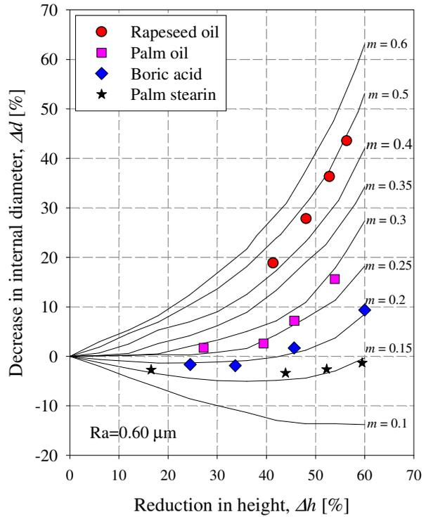
**Fig. 8.** Friction calibration curves and experimental results for the workpiece surface roughness of  $0.60 \mu\text{m}$
