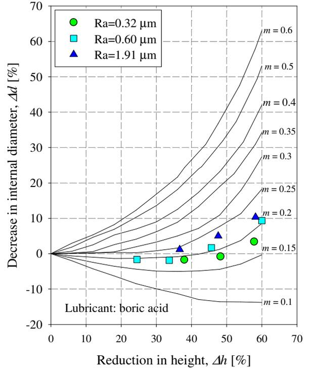
Fig. 12. Friction calibration curves and experimental discrete points in the case of boric acid
