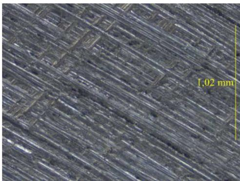
c) - Ring specimen type 3 (Ra=1.91 μm)
