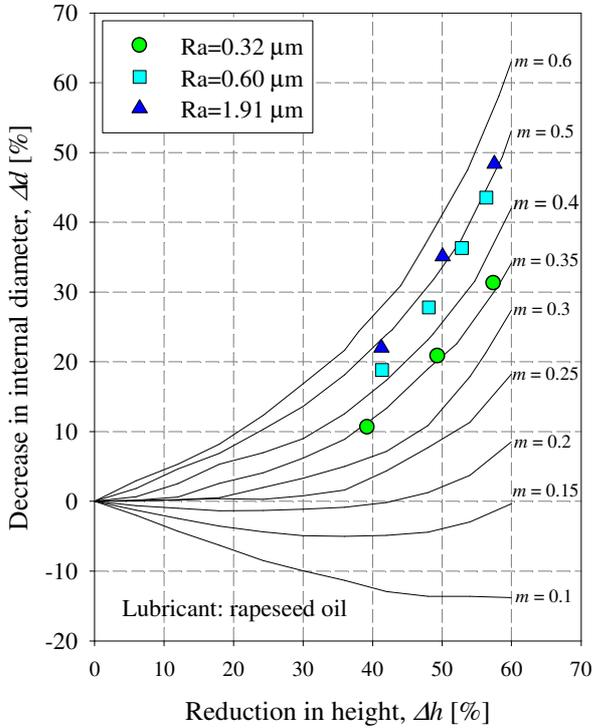
Fig. 10. Friction calibration curves and experimental discrete points in the case of rapeseed oil
