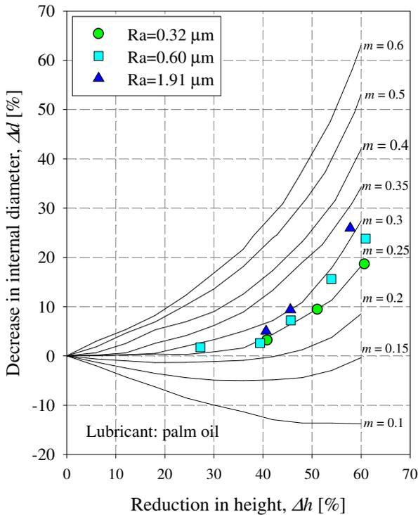
Fig. 11. Friction calibration curves and experimental discrete points in the case of palm oil
