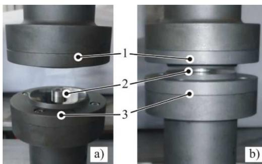
**Fig. 4.** Die setup for ring compression tests
