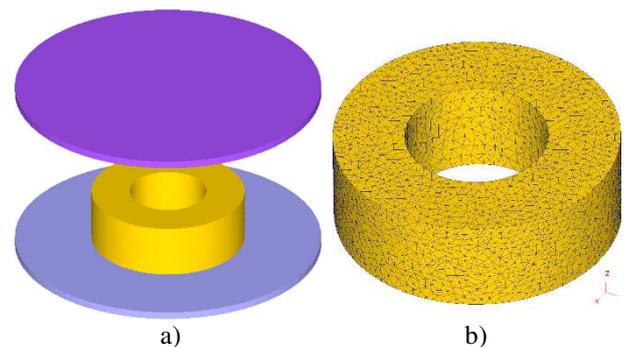
**Fig. 5.** FE simulation of the ring compression test
