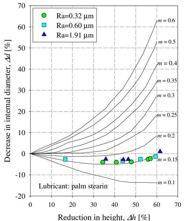
Fig. 13. Friction calibration curves and experimental discrete points in the case of palm stearin
