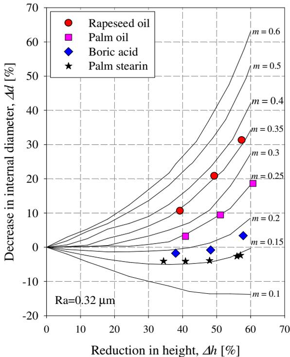
**Fig. 7.** Friction calibration curves and experimental results for the workpiece surface roughness of  $0.32 \mu\text{m}$
