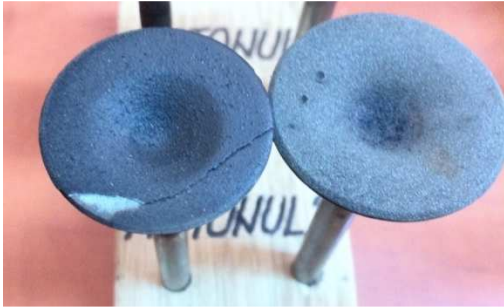
Fig. 12. Valves aspect failure after tests
