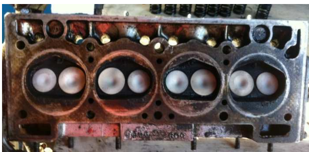
Fig. 8. Operating configurations for S2 ( MgZrO - NiCr ): a) before the tests; b) after the tests (the second row).
