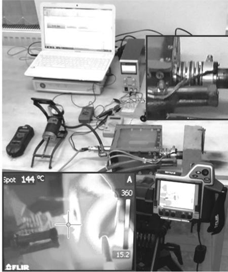
**Fig.4** Experimental installation for determining the power of a Stirling gamma engine according to the working fluid pressure.
