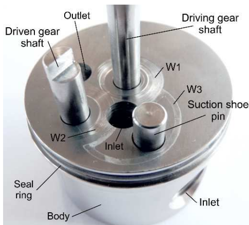
Fig. 3. Worn areas on the micropump body
