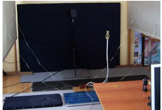
Fig. 11. The whole system for measuring environmental parameters (temperature, luminosity, brightness, noise) [7].
