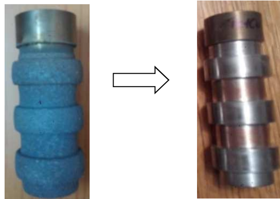
Fig.2. Metallization of the specimen and surface processing
