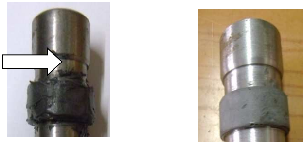
Fig. 5. Using the Loctite Hysol 3478A adhesive on the specimen
