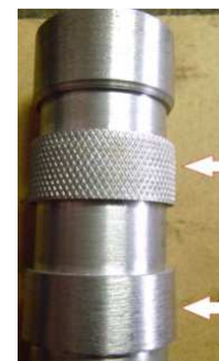
Fig.4. Two possibilities of surface processing with adhesive
