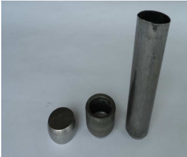
Fig. 5 The sequence of operations at the extrusion of a tubular piece
