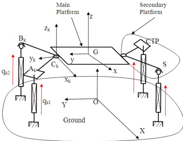
Fig.1. The kinematic scheme of the mechanism
