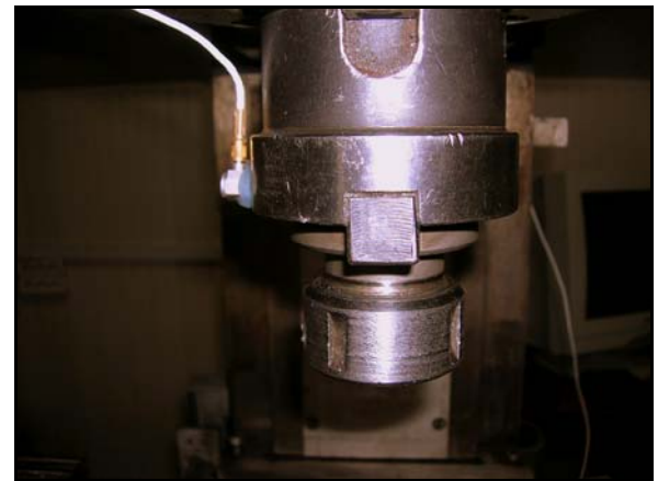
Fig.3 Accelerometer Securing on the main shaft
